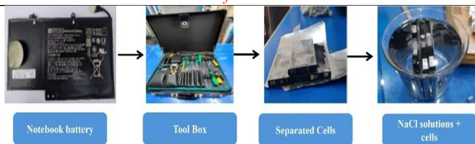
Figure 4. Discharging notebook battery cell
