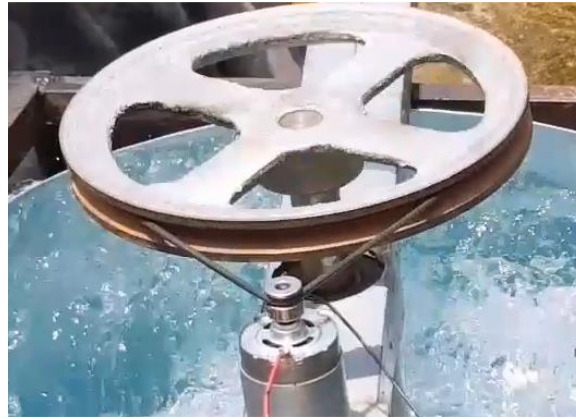
Figure 6. Rope Drive System
