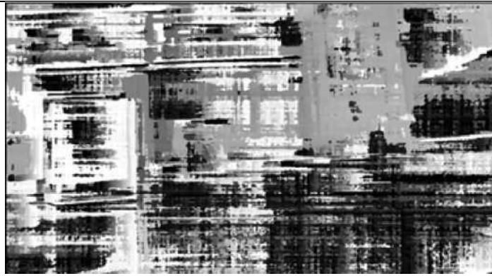
Figure 4. Disparity map without WLS filter
