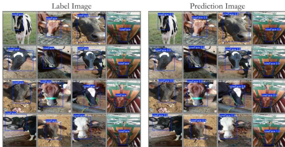
Figure 4. Left: Manually labelled image of cow faces; Right: YOLOv8 prediction of the same image. The model, fine-tuned on a diverse custom dataset, accurately detects cow faces under varying conditions, as shown in the comparison.
