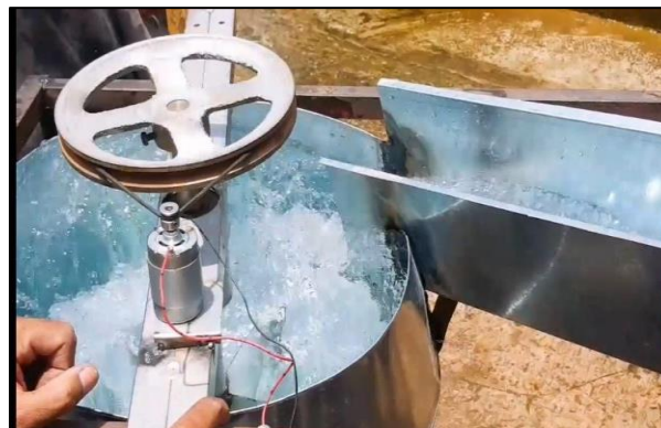
Figure 4. Gravitational water vortex Model
