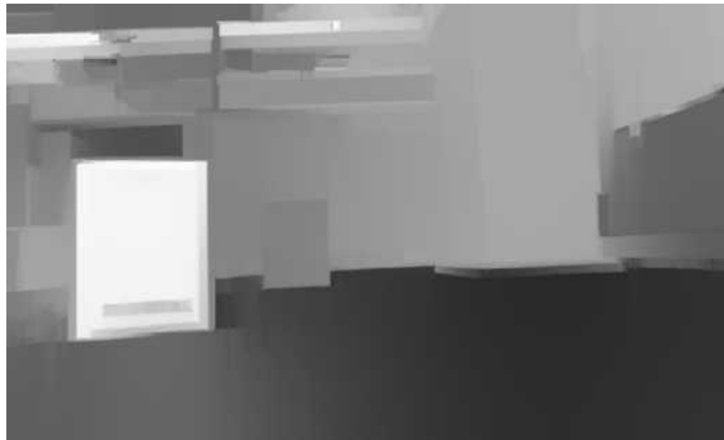
Figure 5. Disparity map after WLS filter
