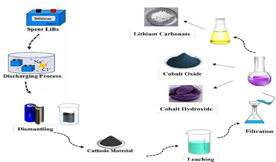
Figure 2. Schematic Diagram of Hydrometallurgical recycling procedure
