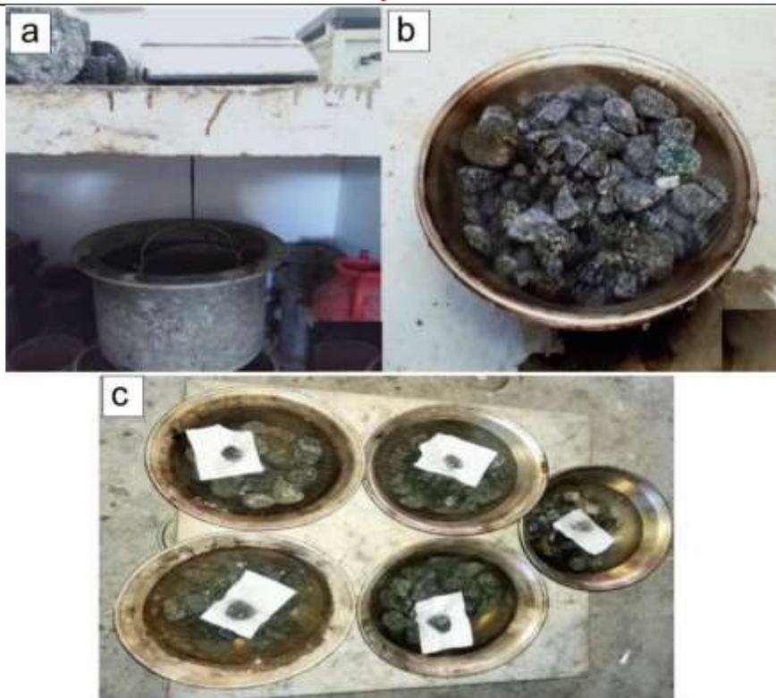
**Figure 5.** a) Weighing in water procedure, (b) Aggregates dipped in water as per ASTM standards, (c) Demonstrating the soundness test procedure for granite rock aggregates, with samples immersed in a water vessel containing  $MgSO_4$  solution.
