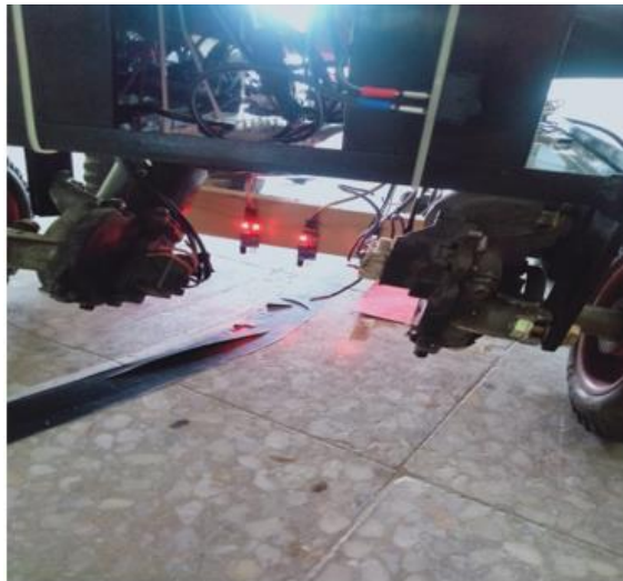
Figure 22. Destination Detection Using Color Sensor
