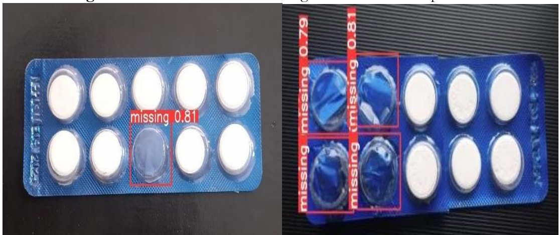
Figure 16. (a) Results show a missing tablet with a Rectangular Red Box. (b) Results showing four missing Tablets in the Blister Strip
