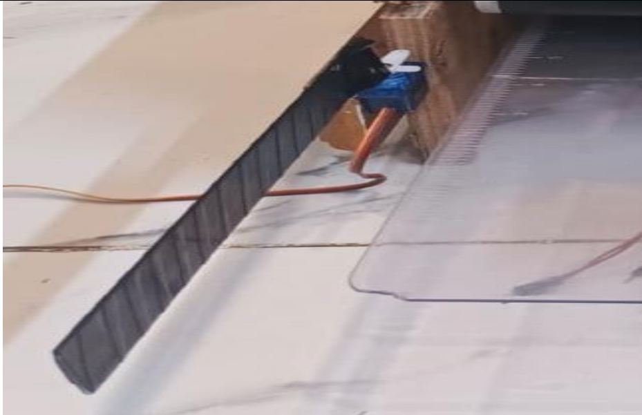
Figure 22. Servo Motor with a removing bar
