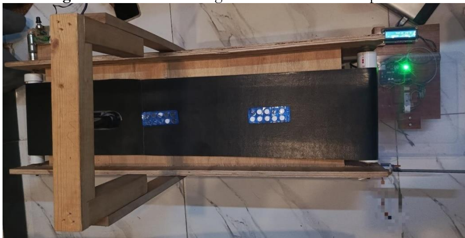
Figure 18. Real-time detection of defects by the Tablet Guard System
