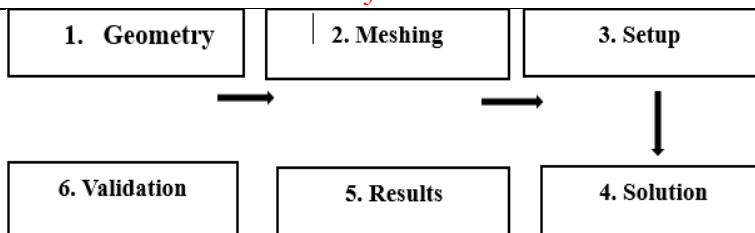
Figure 6. Flow diagram of methodology of the process used for the degradation in CFD simulation
