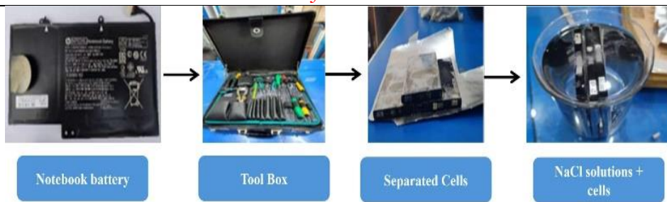
Figure 4. Discharging notebook battery cell
