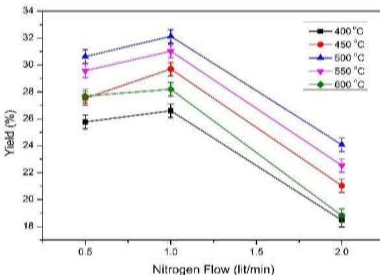
**Figure 5.** Nitrogen Flow's impact on Bio-oil Yield %
