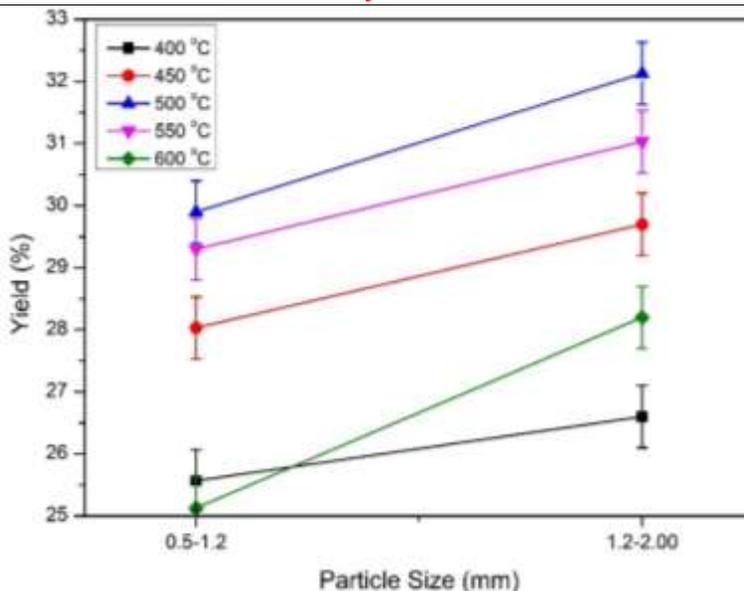
**Figure 4.** Particle Size's impact on Bio-oil Yield %
