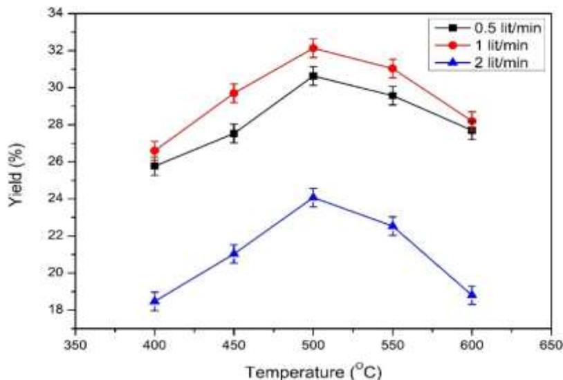
**Figure 3.** Temperature's impact on Bio-Oil Yield %
