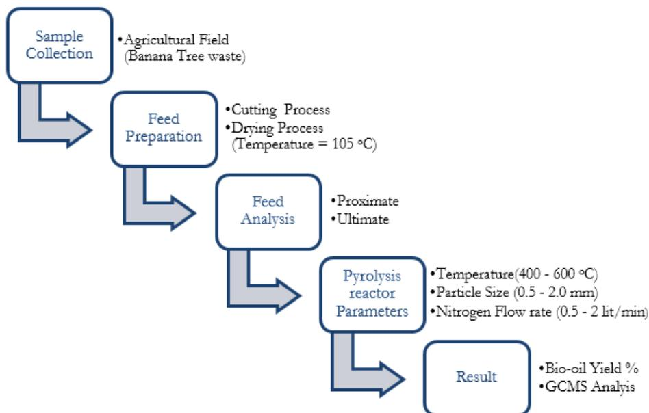
**Figure 2.** Flow diagram of Pyrolysis process
