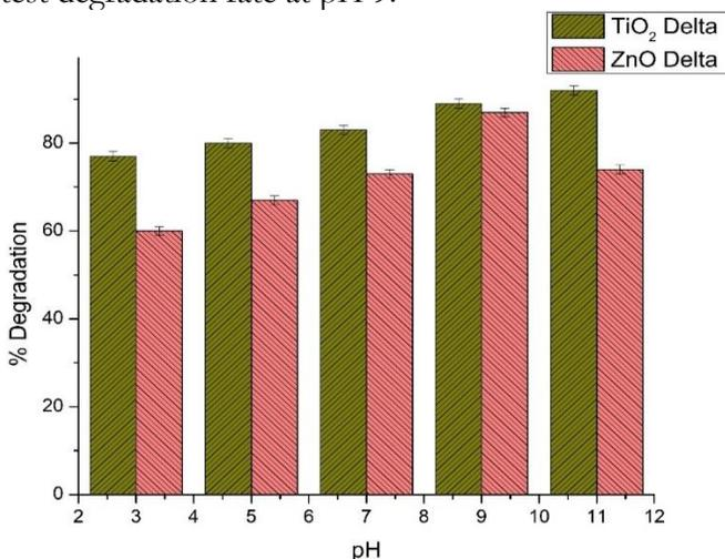
**Figure 6.** The efficiency of degradation at different pH of Deltamethrin Sample with ZnO and TiO<sub>2</sub>
