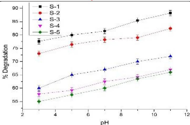
**Figure 2.** Efficiency of degradation at various pH of Deltamethrin Samples with TiO<sub>2</sub> Catalyst: Different Dosing and Degradation Efficiency
