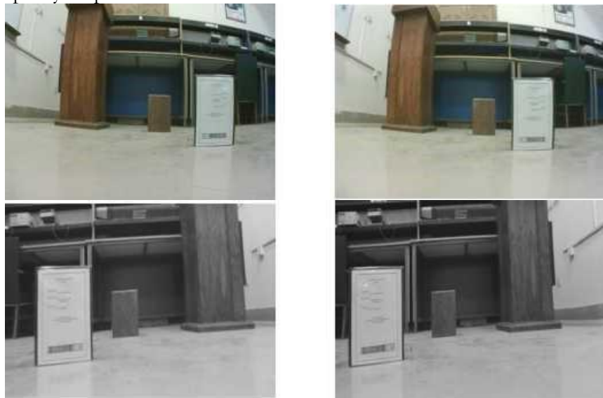
Figure 3. Left and right images before and after rectification
