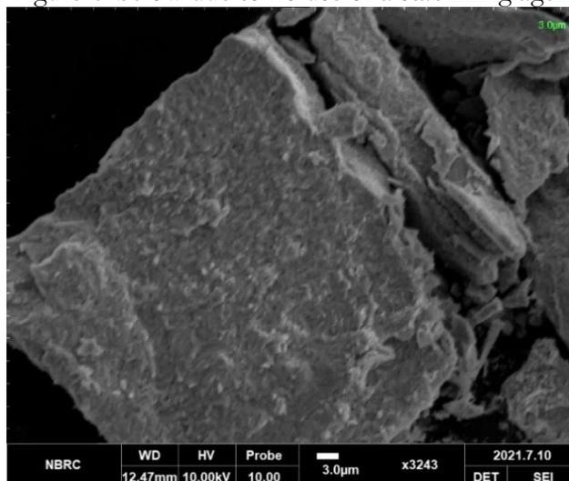
**Figure 4.** Scanning electron microscope (SEM) analysis nanoparticles synthesized by *Serratia marcescens* w2 strain showing the obtained nanoparticles are nonporous and non-uniform.
