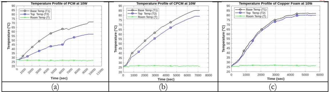
Figure 6. Temperature Profile at 10W of (a) PCM (b) CPCM (c) Copper Foam
