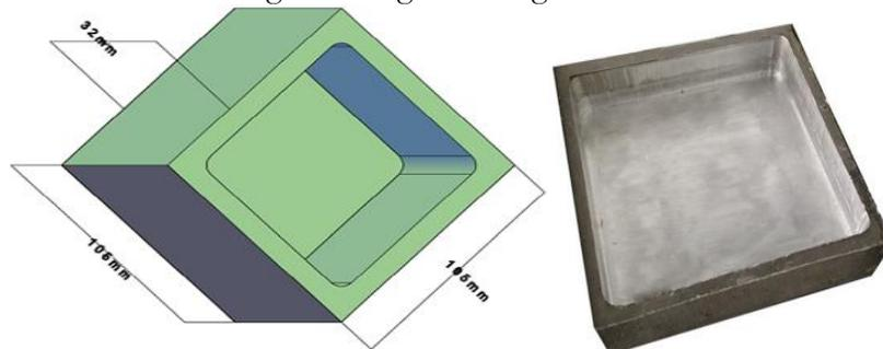
**Figure 4.** Heat Sink with its dimensions
