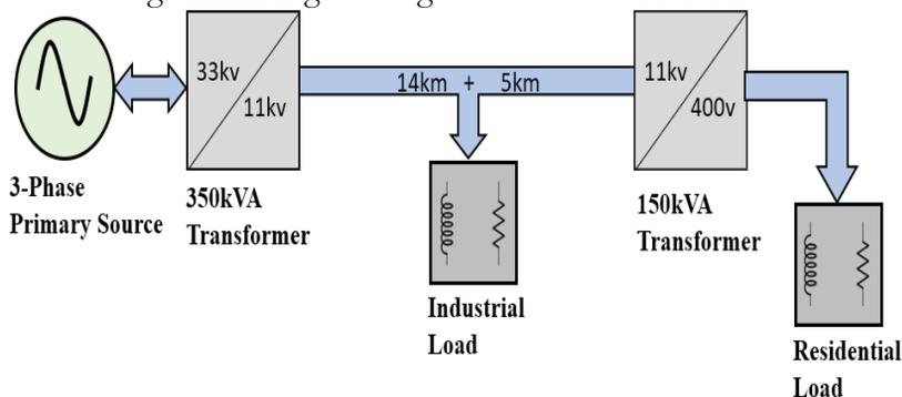
**Figure 2.** Block diagram of the distribution grid
