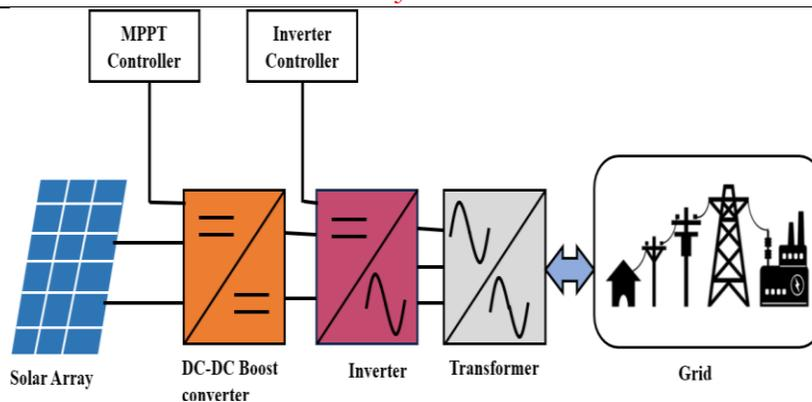
**Figure 1.** Block diagram microgrid integration of a PV fed with the distribution grid
