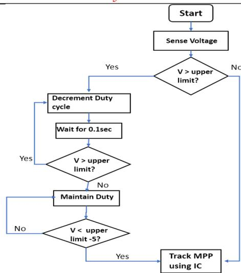
**Figure 4.** Flowchart of Modified Incremental Conductance method
