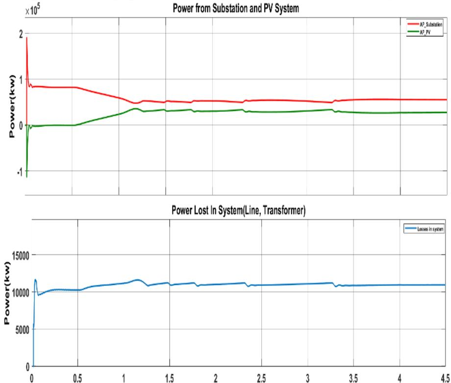
Figure 6. Power profile without the proposed IC method
