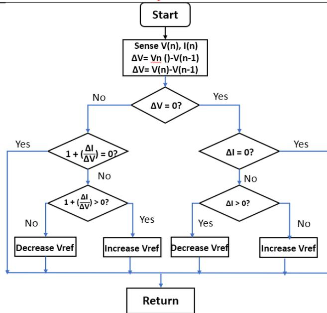
Figure 3. Traditional Incremental Conductance Flowchart
