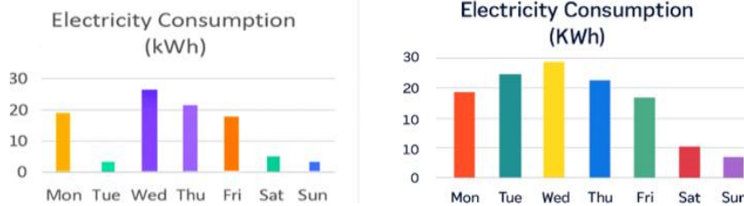
Figure 2. Daily Electricity Consumption (a) Low consumption during weekends is normal; (b) Low consumption during normal weekdays is anomalous.
