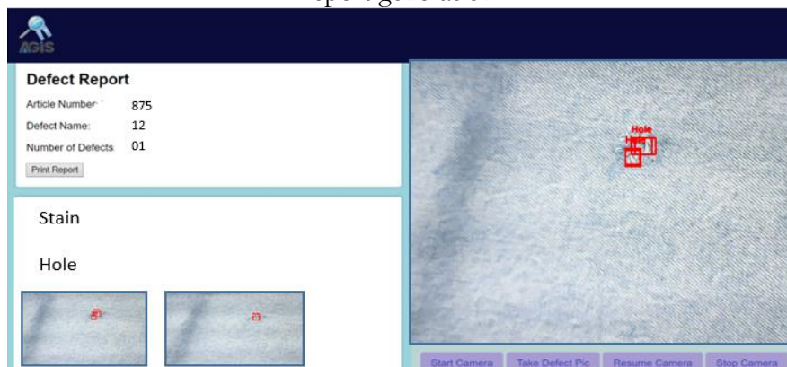
Figure 8(B). Representation of User Interface: Real-time defect detection of holes and report generation.
