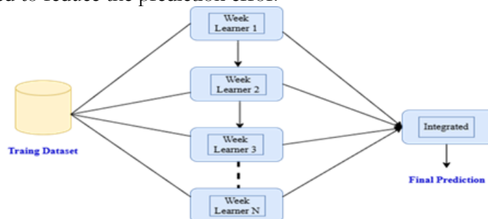
Figure 3. Working Mechanism of the Ensemble Method: Gradient Boost
