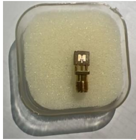
Figure 2. Fabricated design of T-shaped slot patch antenna
