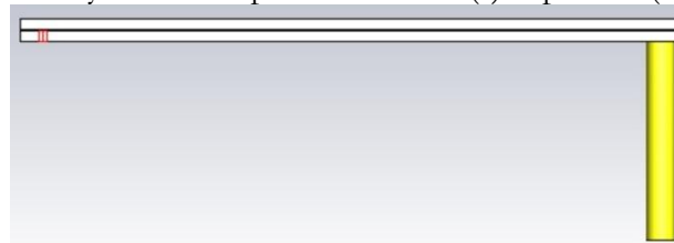
Figure 3. Probe-Fed and Shorting Pin Side View
