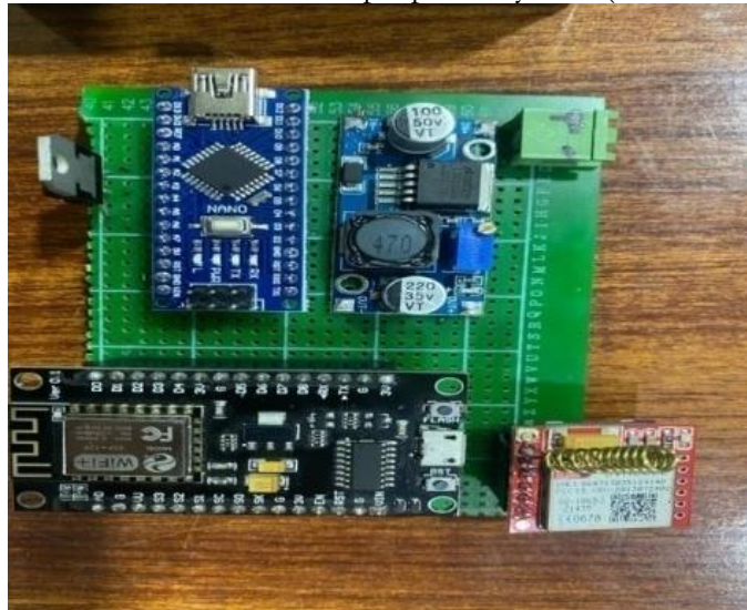
Figure 2. Hardware prototype of the proposed car battery theft prevention system
