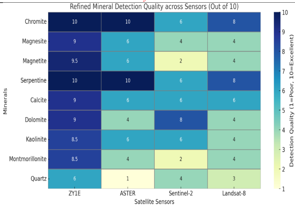
Figure 14. Overall minerals detection performance of all sensors.
