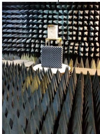
Figure 13. Measurement setup of a proposed MIMO antenna in an anechoic chamber (on a turntable).
