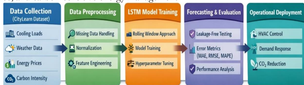
Figure 6. Overall workflow of the proposed leakage-free LSTM-based forecasting framework, illustrating data collection, preprocessing, model training, evaluation, and operational deployment for short-term cooling demand prediction.
