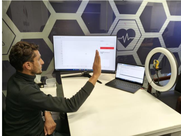
Figure 2. Image of the experimental setup showing the RD-03D radar mounted on a tripod facing a subject performing a hand gesture.
