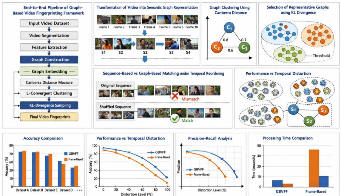
Figure 3. End-to-end architecture of the proposed Graph-Based Video Fingerprinting Framework (GBVFF), illustrating the transformation from raw video input to final graph-based fingerprints used for retrieval and matching.
