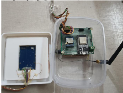
Figure 3. System prototype setup (RFID reader – MCU – LoRa transmitter)
