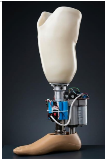
Figure 1. The developed powered ankle prosthesis on which the flex sensor subsystem is integrated. The self-contained module mounts distal to the prosthetic socket and contains the linear actuator, microcontroller, sensing electronics, and battery, with the flex sensor mounted across the knee region of the socket.
