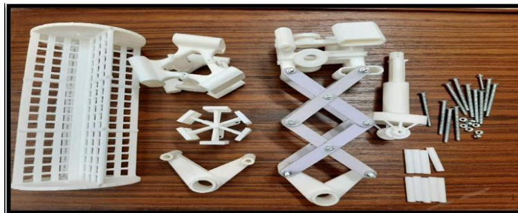
Figure 13. Body of the robot manufacture by PLA (3D printing).
