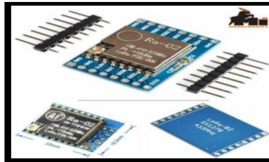
Figure 11. LoRa (SX1278 Module)
