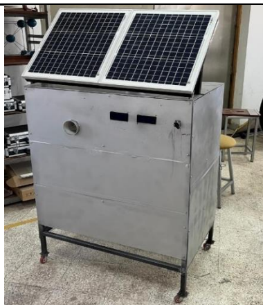
Figure 5. Completed air purifier prototype with dual solar panels, LCD display, and outlet duct
