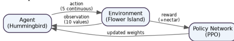
Figure 2. The reinforcement-learning interaction loops between the agent, its policy, and the environment
