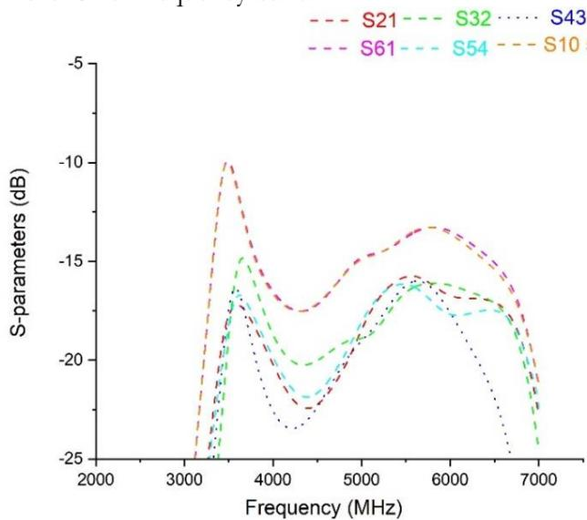
Figure 5. S-parameters: Transmission coefficients of the proposed MIMO antenna.
