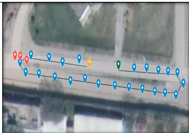
Figure 11 Final testing on a complete path with points representing followed path and line representing path to be followed.
