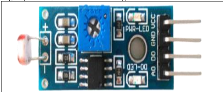
Figure 8. The picture was taken on the white background of LDR Module LM 393 used for light sensing
