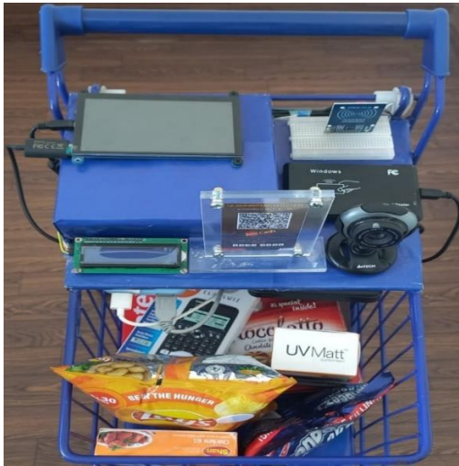
Figure 6: Autonomous Trolley with Smart Billing
