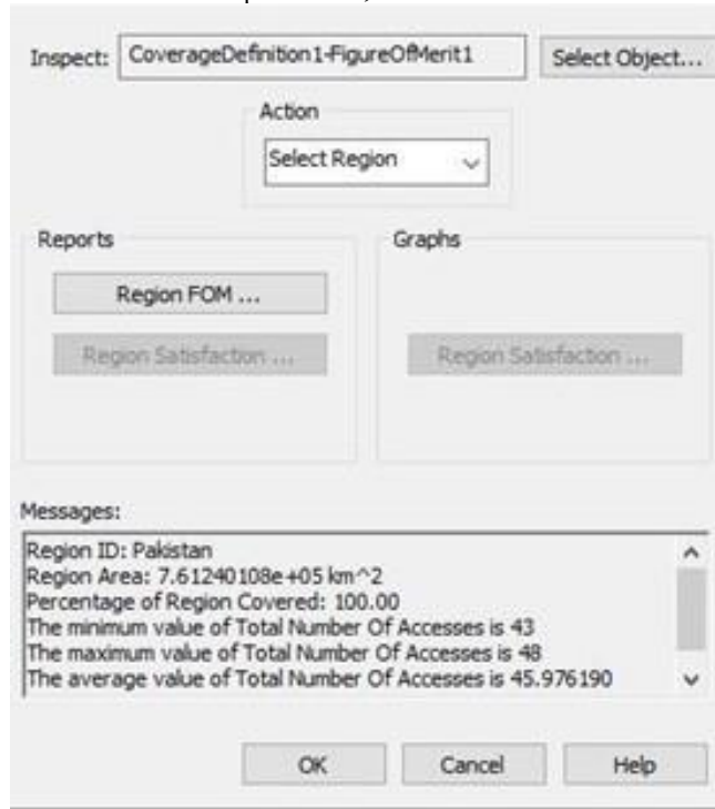
Figure 8: STK window showing the figure of merit for satellite accesses over Pakistan with six satellite constellations.
