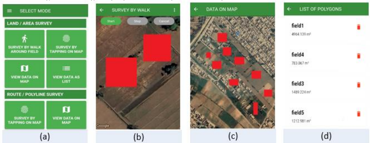
Figure 3: (a) Main menu of application (b) Polygon drawn by tapping (c) View of survey data on map (d) List view of collected data
