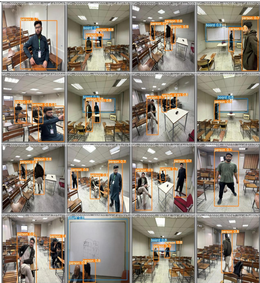
Figure 5. Test images showing the object detection of board and students as a person
