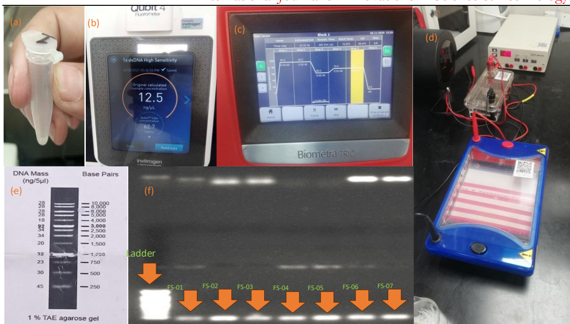
Figure.7. Molecular Identification of fungal species: FS-01 to FS-07 a Extracted DNA b Concentration of DNA c PCR Amplification d Agarose gel electrophoresis e 1kb base pair of 1% TAE agarose gel f DNA fragment and PCR Product on UV gel studio SA 2 .
