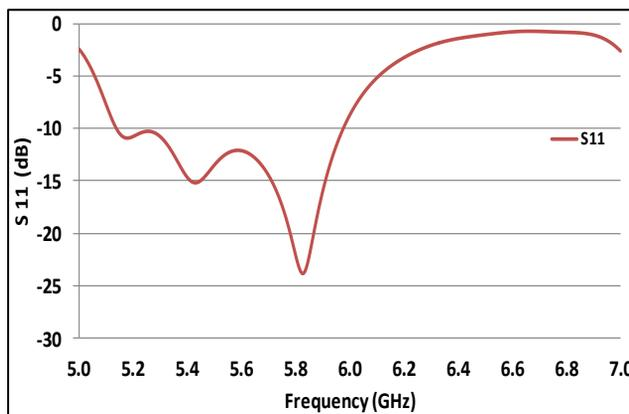
Figure 7: Reflection coefficient (S11) of proposed antenna
