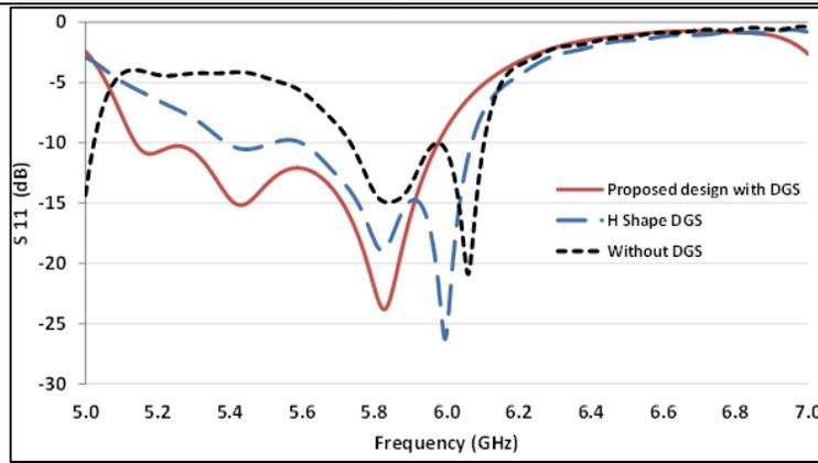
**Figure 8:** Simulated S11 of proposed Antenna and without DGS Structure.
