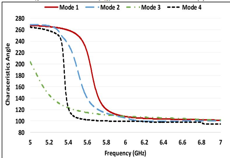
Figure 5: Characteristics mode analysis Mode 1-4
