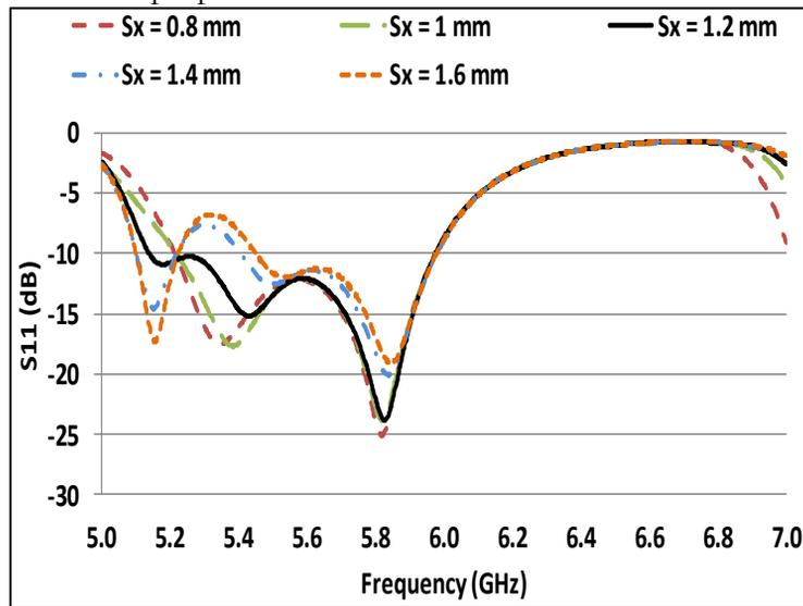
**Figure 9:** Parametric sweep of DGS Structure on  $S_x$ .
