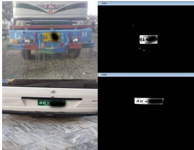
Figure 2. (a) Input image with yellow plate, (b) Mask image, (c) Input Image with green Plate and (d) Mask image
